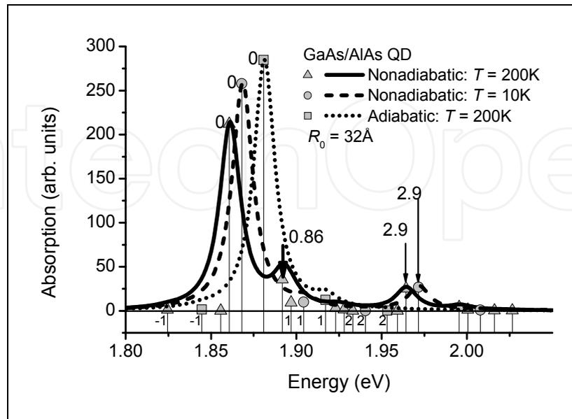
Fig. 5. Simulated absorption spectra of GaAs/AlAs nanocrystal QDs.
