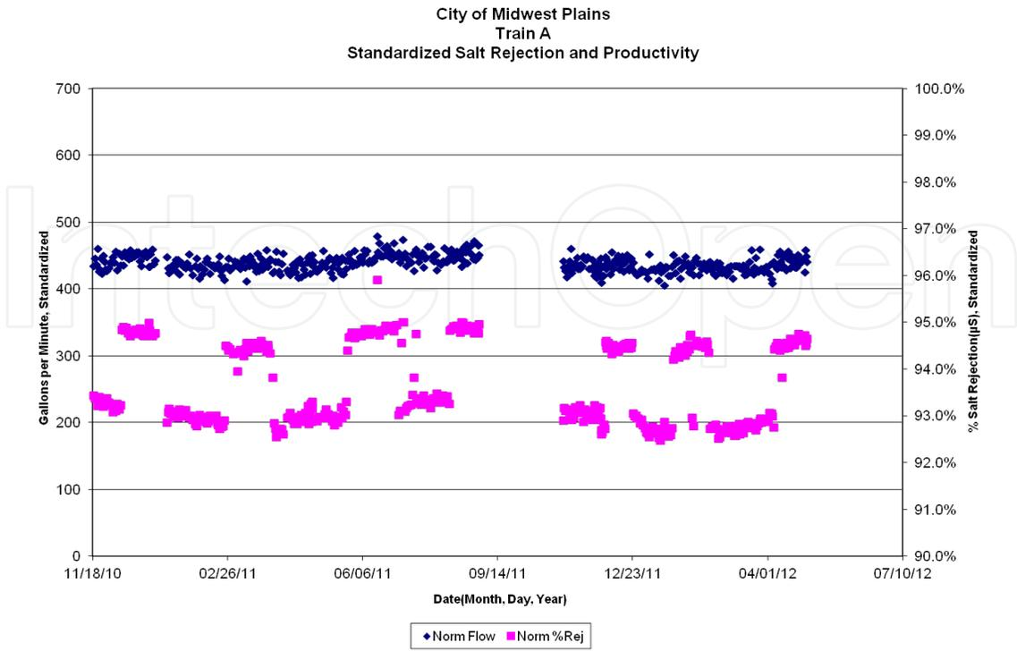
Figure 2. Standardized System Data: Permeate Productivity and Salt Rejection.
