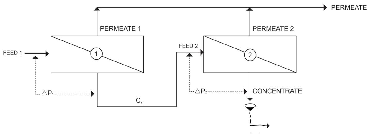
**Figure 1.** Medium and larger membrane systems are organized into multiple stages, usually two stages.
