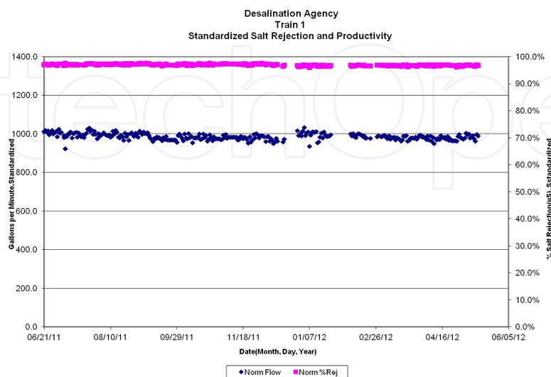
Figure 4. Normal Fouling and Salt Rejection.
