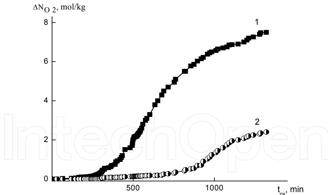
Fig. 1. The kinetic curve of oxygen absorption PP (1), and PE (2)  $T_{\text{ox}} = 110^\circ\text{C}$ ,  $p_{\text{O}_2} = 600 \text{ mm Hg}$
