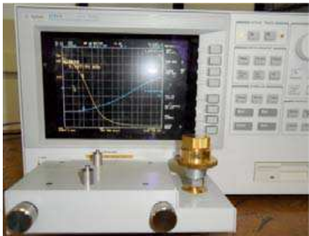
Fig. 9. Impedance meter Agilent 4294A and magnetic module
