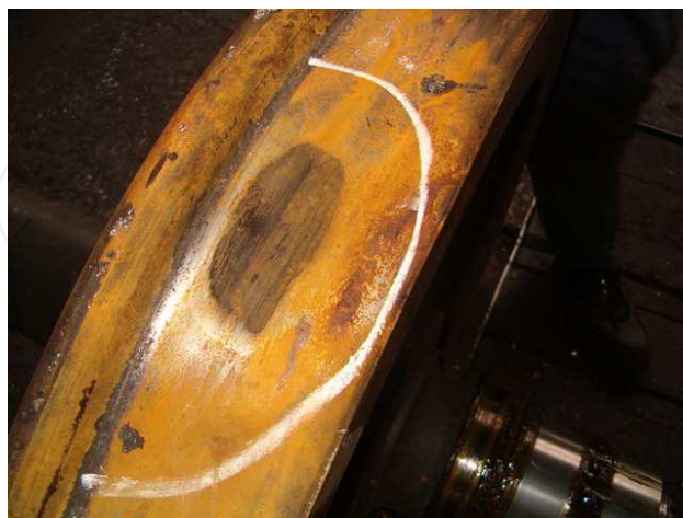
Fig. 2. Flat spot on a wheel tread 2
