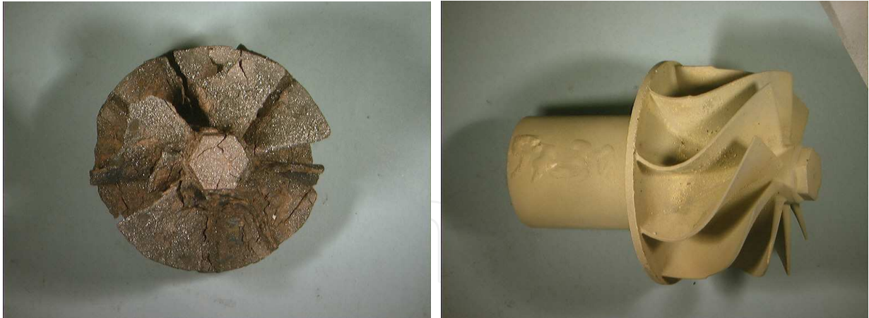
Fig. 23. Turbocharger rotor manufactured from a \gamma -TiAl-alloy after oxidation for 1000 h at 1050°C in air. Left image: Untreated rotor. Right image: Fluorine-treated rotor.
