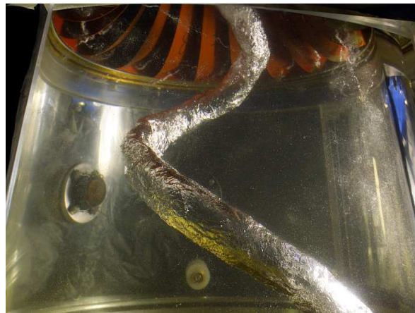
Fig. 2. Development of a cavitating helical vortex downstream the runner of a Francis turbine at partial load
