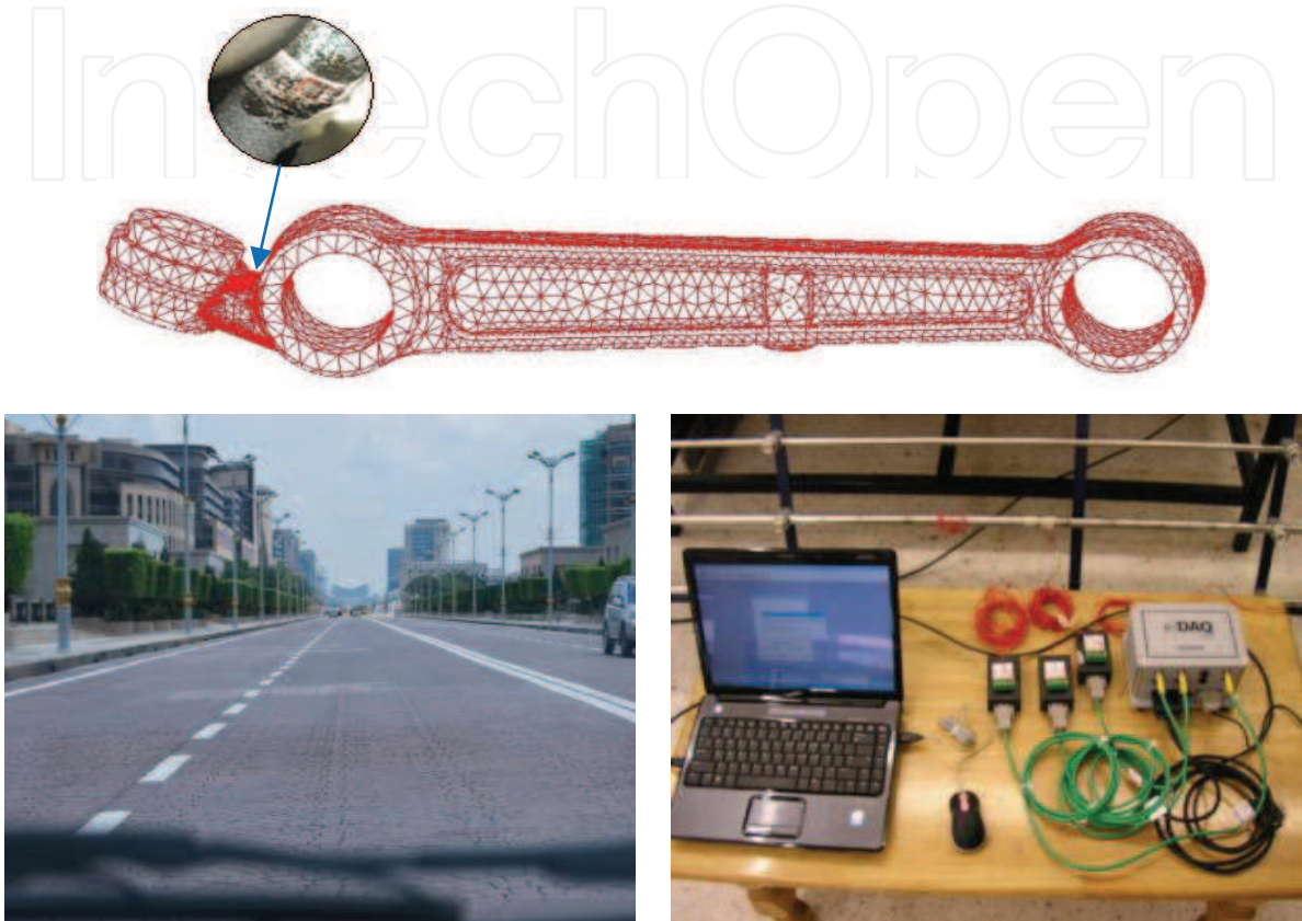
Fig. 2. The strain gauge position, a section of the pavé test track and the data acquisition set-up
