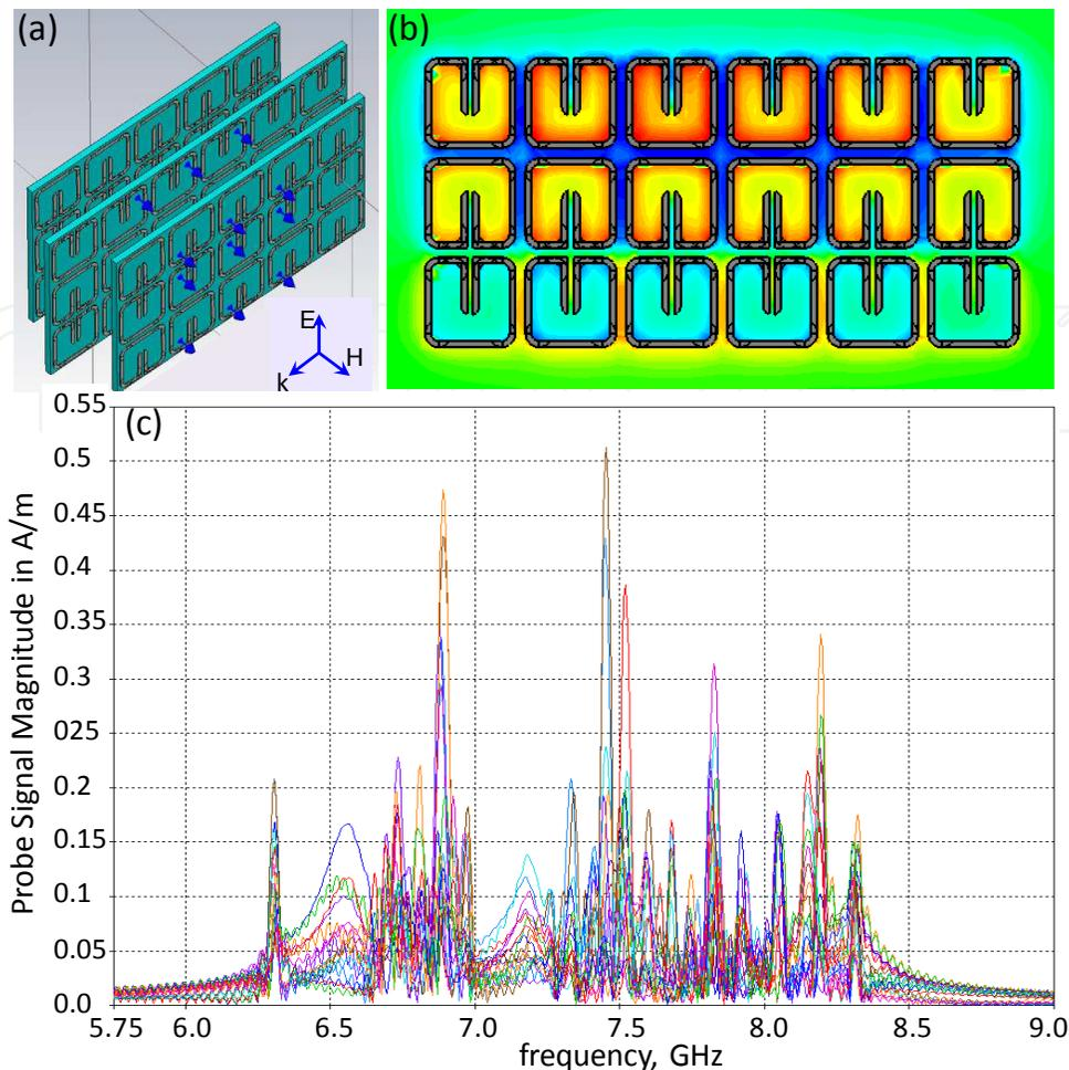
Fig. 8. (a) Geometry of a three-layer SRR array with marked probe locations; (b) coherent response of SRRs at 8.35 GHz; and (c) spectra of probe signals revealing enhanced splitting caused by interaction between SRRs in neighbouring layers.
