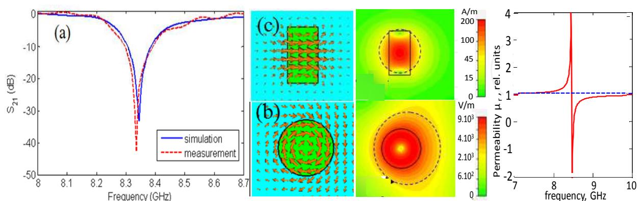
Fig. 9. (a) Simulated and measured  $S_{12}$  spectra for a DR in WR137; (b) electric and (c) magnetic field patterns in DR cross-sections; and (c) effective permeability changes at the magnetic-type resonance in the DR (Chen et al., 2011).
