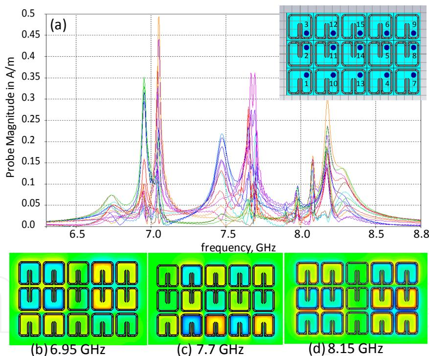
Fig. 6. (a) The spectra of the probe signals; inset shows the SRR array and the H-field probe locations; (b)-(d) typical patterns of the resonance oscillations in the array sampled at 6.64, 7.4 and 8.15 GHz (colour intensity shows the magnitude of resonance oscillations).
