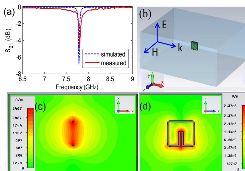
Fig. 2. Resonance in a single SRR placed in the waveguide WR137: (a) measured and simulated transmission spectra  $S_{21}$ ; (b) arrangement for the measurements; (c) magnetic and (d) electric field patterns.
