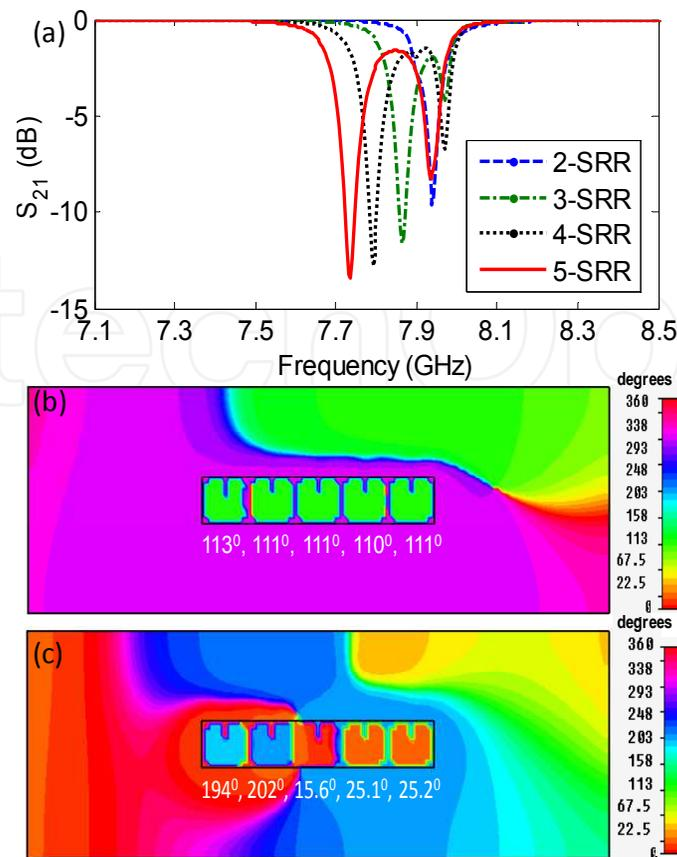
Fig. 3. Resonances in linear arrays arranged in wave propagation direction in the waveguide WR137: (a)  $S_{21}$ ; (b) coherent response of a 5-SRR array at 7.73 GHz; and (c) asymmetric response at 7.95 GHz.
