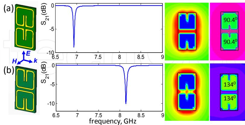
Fig. 5. Geometry,  $S_{21}$  spectra, and patterns of H-field magnitude (3<sup>d</sup> column) and phase (4<sup>th</sup> column) for SRR pairs arranged: (a) “face-to-face” and (b) “back-to-back”.
