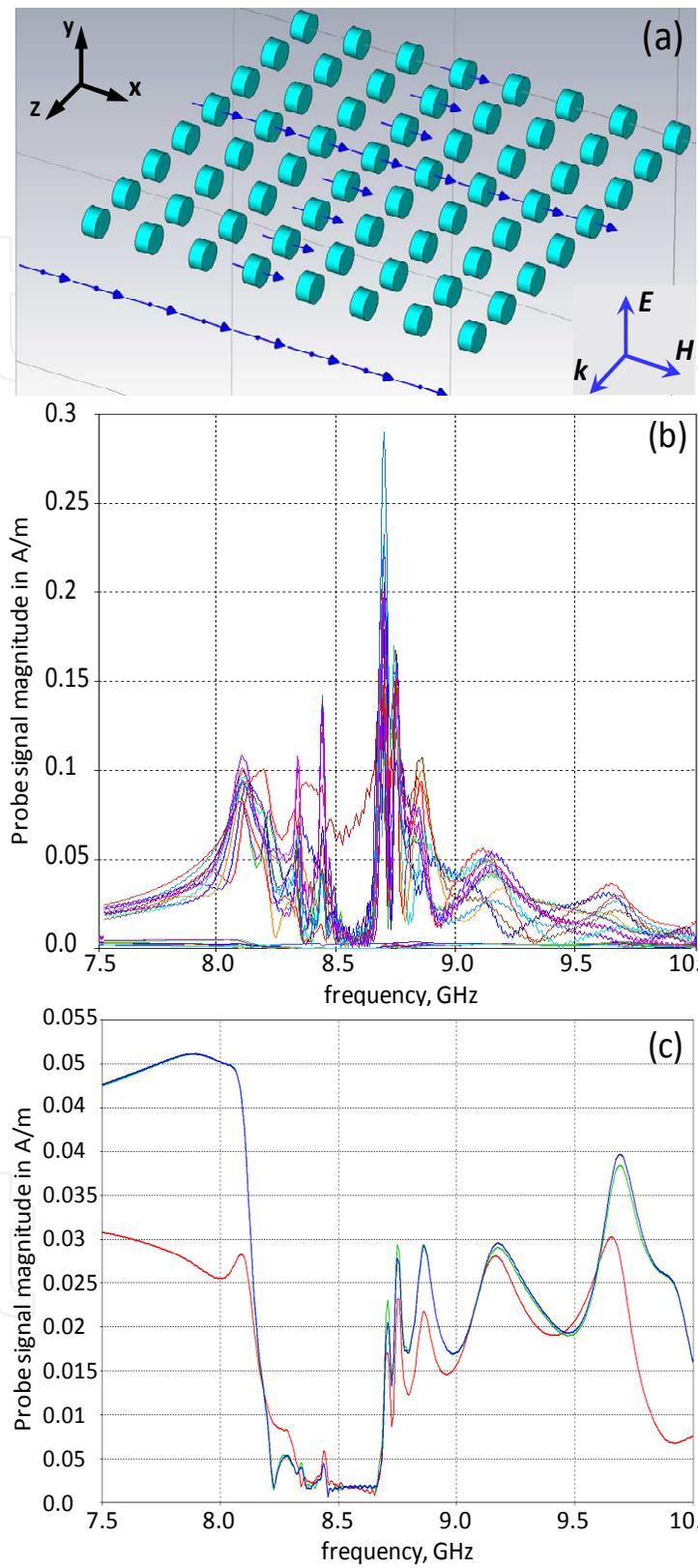
Fig. 14. (a) Basic element of 3D arrays at plane wave incidence in  $z$ - and PBC in  $y$ -direction; (b) spectra of signals from probes placed in DR centres; and (c) spectra of probes placed outside the sample to detect transmission.
