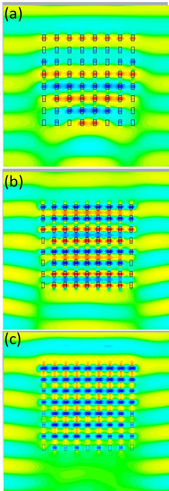
Fig. 15. Wave propagation in 3D DR arrays at frequencies (a) below the gap and (b, c) above the gap at: (a) 8.0 GHz; (b) 8.74 GHz; and (c) 8.64 GHz.
