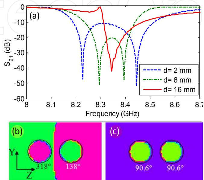
Fig. 11. (a)  $S_{21}$  spectra for two DRs arranged along the axis of the waveguide WR137; (b) and (c) phase patterns for H-field distributions in the longitudinal cross-section at 2 split resonances (Chen et al., 2011).
