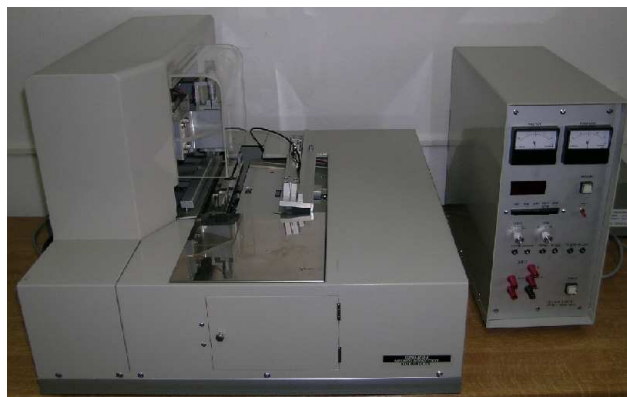
Fig. 1. Device for measurement of fabric surface characteristics
