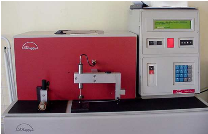
Fig. 5. The step thickness meter SDL M 034/1
