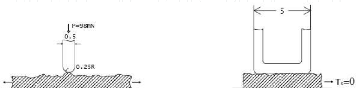
Fig. 2. KES contactor for measuring of surface roughness
