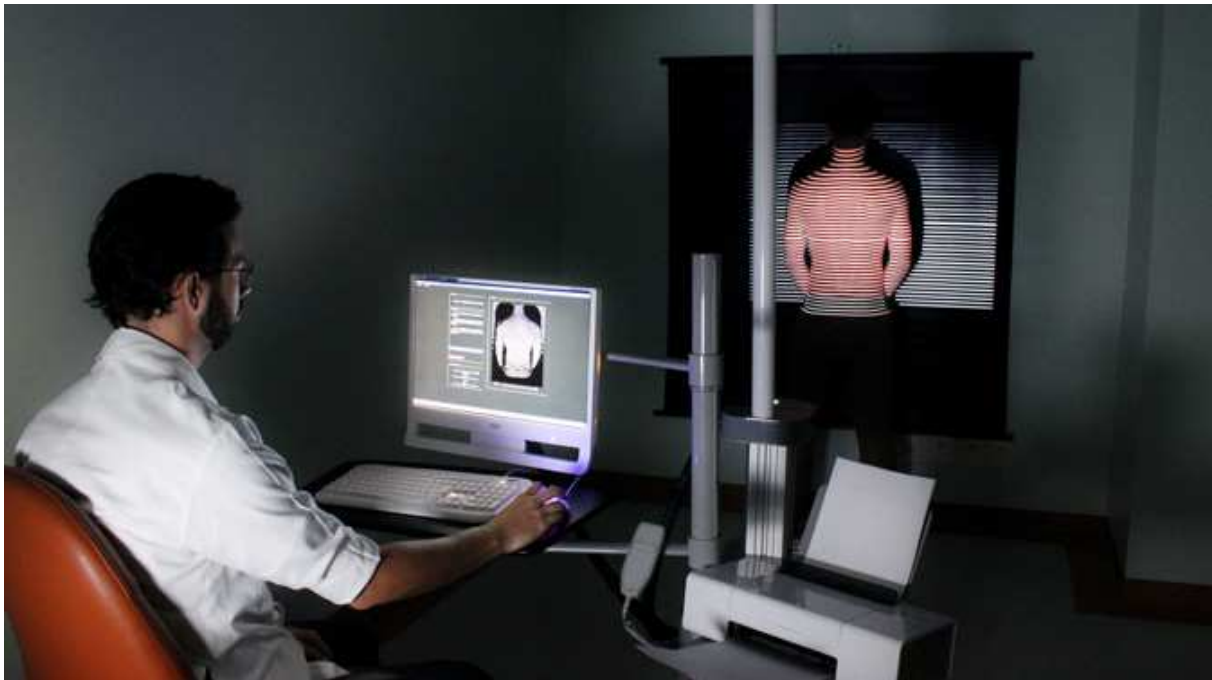
Fig. 2. Projection Moiré Technique. From: www.miotec.com.br .
