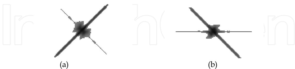
Fig. 25. Image of simple line segments filtered using (a) a rotated elliptic Gaussian filter with forward estimation, and (b) a rotated elliptic Gaussian filter with inverse estimation.
