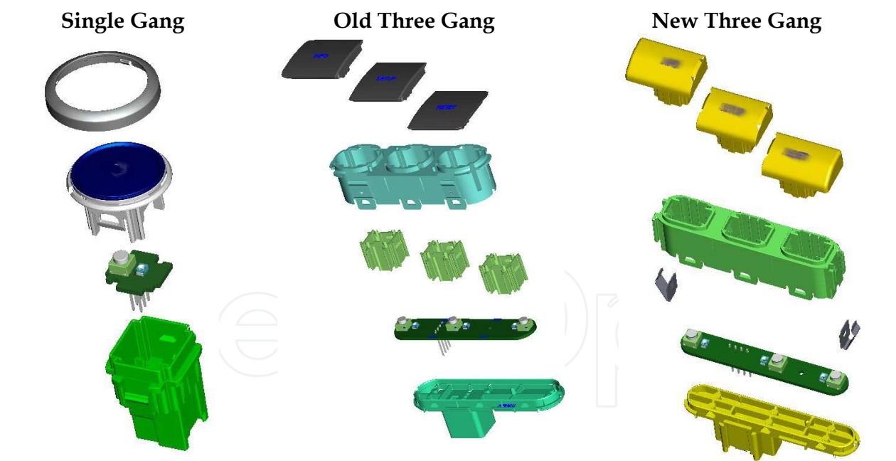
Fig. 1. An exploded view of a representative member of each product family
