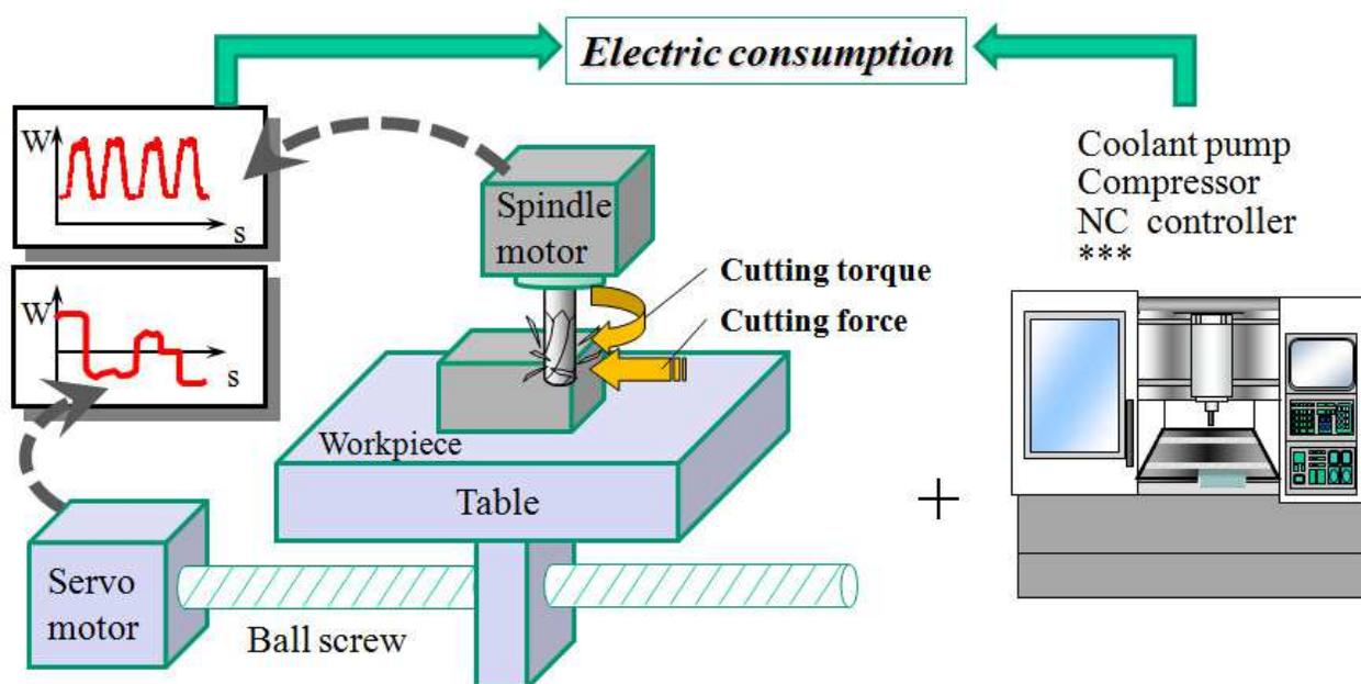
Fig. 2. Electric consumption model for machine tool
