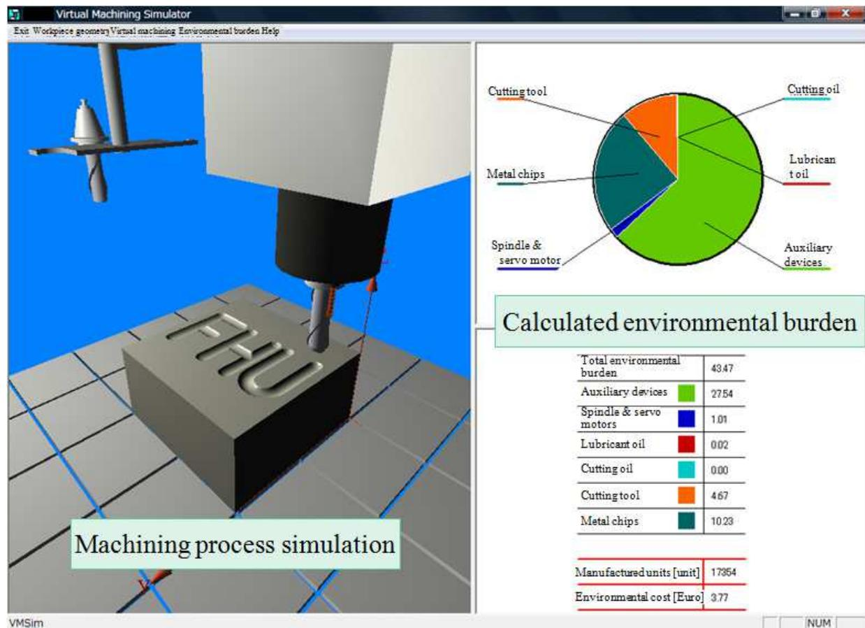
Fig. 3. An output example of the developed analyzer
