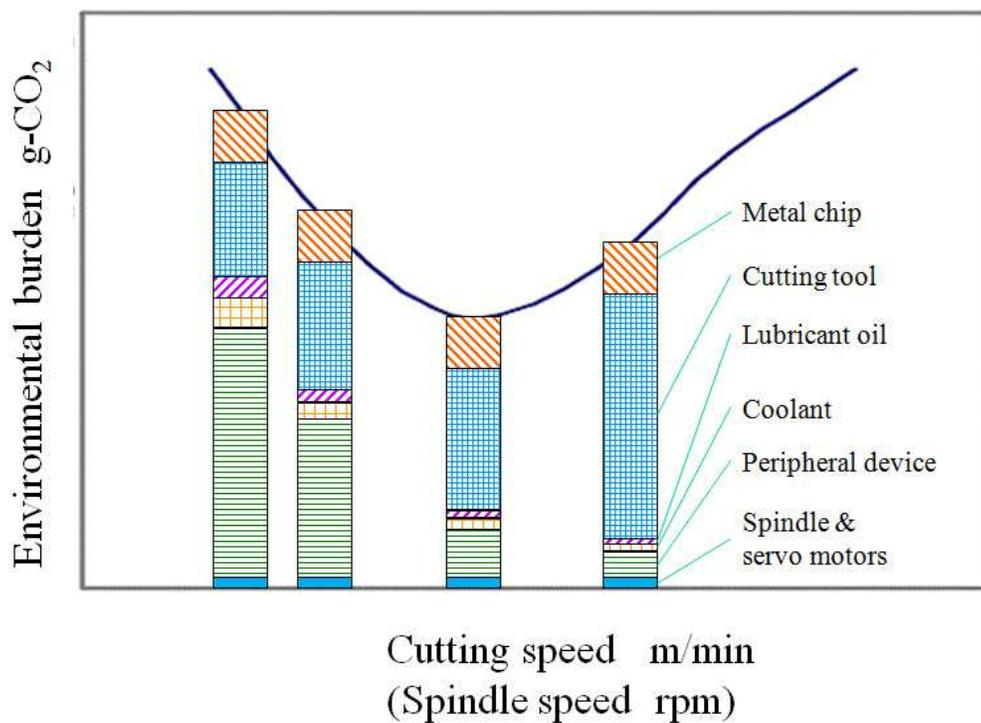
Fig. 6. Tendency due to high speed milling
