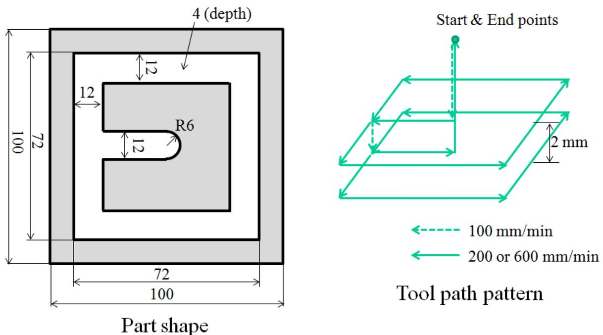
Fig. 4. Part shape and tool path pattern
