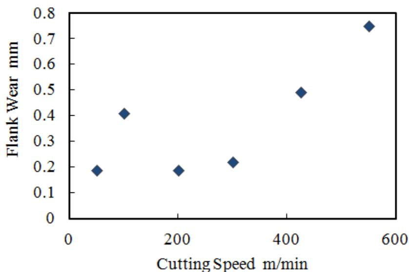
Fig. 7. Tool wears according to cutting speed (Anzai, 2003)
