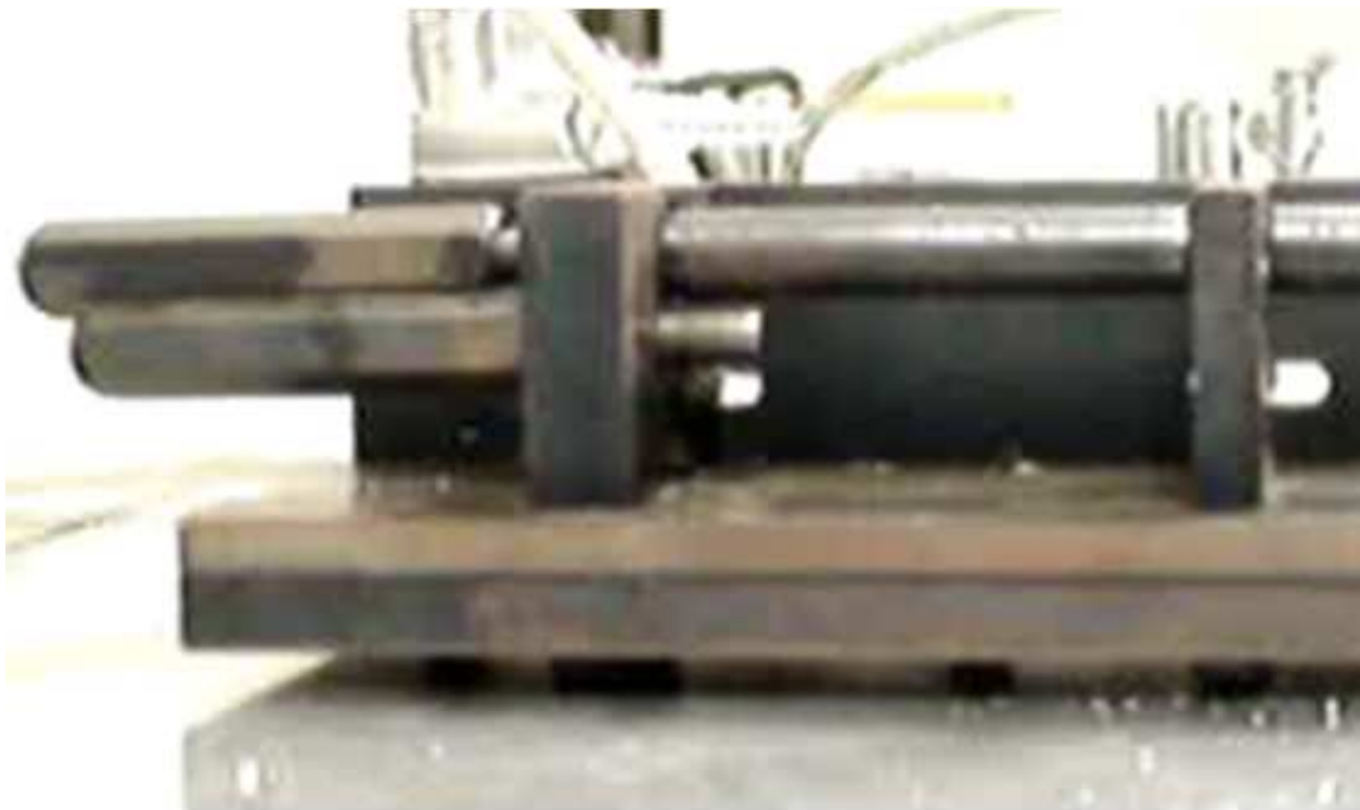
Fig. 24. Pin element changes height.
