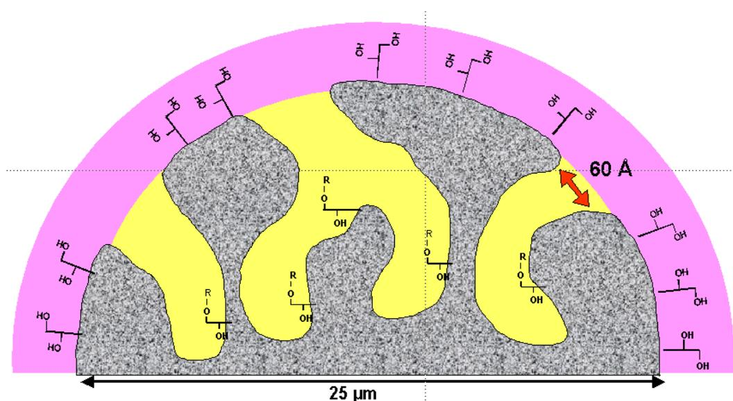
Fig. 3. Artistic representation of a SCX-RAM silica particle (LiChrospher 60 XDS (SO<sub>3</sub>/Diol), Merck KGaA, Germany). The external surface is coated with hydrophilic, electroneutral diol-groups for the exclusion of high molecular weight components (>15 kDa); the internal surface is functionalized with ion-exchange groups accessible for low molecular weight components which may be trapped by electrostatic interaction.
