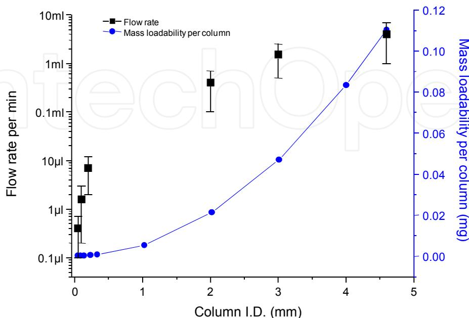
Fig. 6. Estimation of monolithic silica columns flow rates and mass loadability per column. Columns 2, 3 and 4.6 mm I.D. are 10 cm long; columns 50  $\mu\text{m}$ , 100  $\mu\text{m}$  and 200  $\mu\text{m}$  are 15 cm long.
