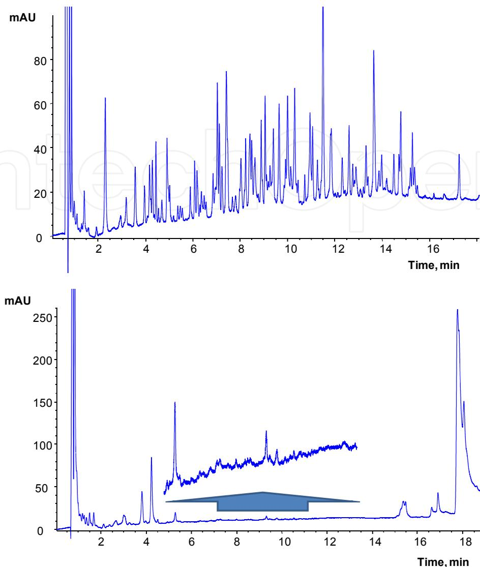
Fig. 2. Separation of standard protein digest and real biological sample analysis: upper chromatogram - 1  $\mu$ l BSA digest (1mg/ml), lower chromatogram 8  $\mu$ l of filtered amniotic fluid. Conditions: column - Chromolith Performance RP-18e 100 mm  $\times$  2 mm I.D.; eluents - A: 95% H<sub>2</sub>O/5% ACN/0.1% TFA (v/v/v), B: 5% H<sub>2</sub>O/95% ACN/0.085% TFA (v/v/v); gradient - from 5% B to 50% B in 20 min; flow rate - 0.3 ml/min, detection - UV 214 nm.
