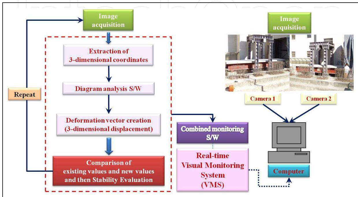
Fig. 1. Analysis procedure of VMS using digital photogrammetry
