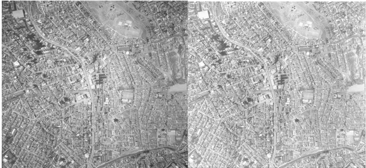
Fig. 14. Correction of vignetting effect of left image showed in the right.
