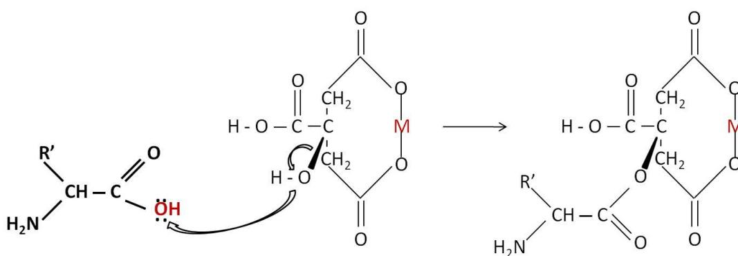
Fig. 2. Synthesis mechanism of the modified Pechini method.
