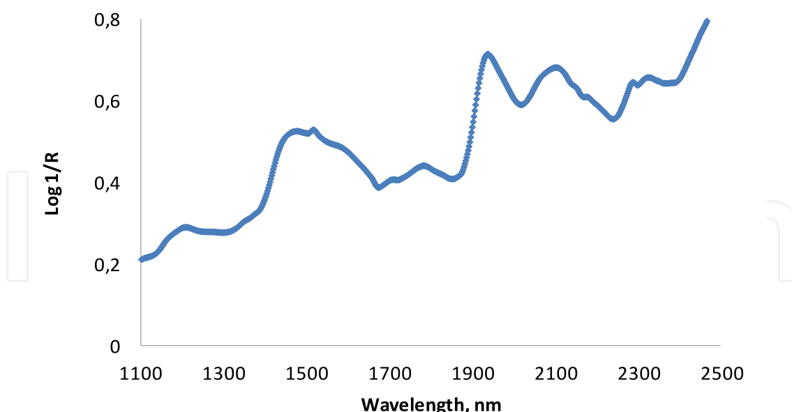
Fig. 1. NIR reflectance spectrum of wheat flour (1100-2500 nm) recorded by FOSS's NIRSystem 6500
