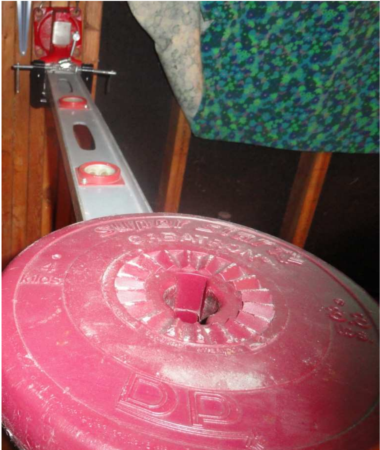
Fig.3. Weight placed on the beam 0.9 m (3 ft) from the vise
