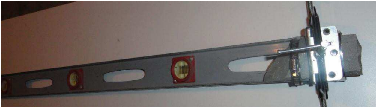
Fig.2. Metal Extension attached to the CWF2 Beam
