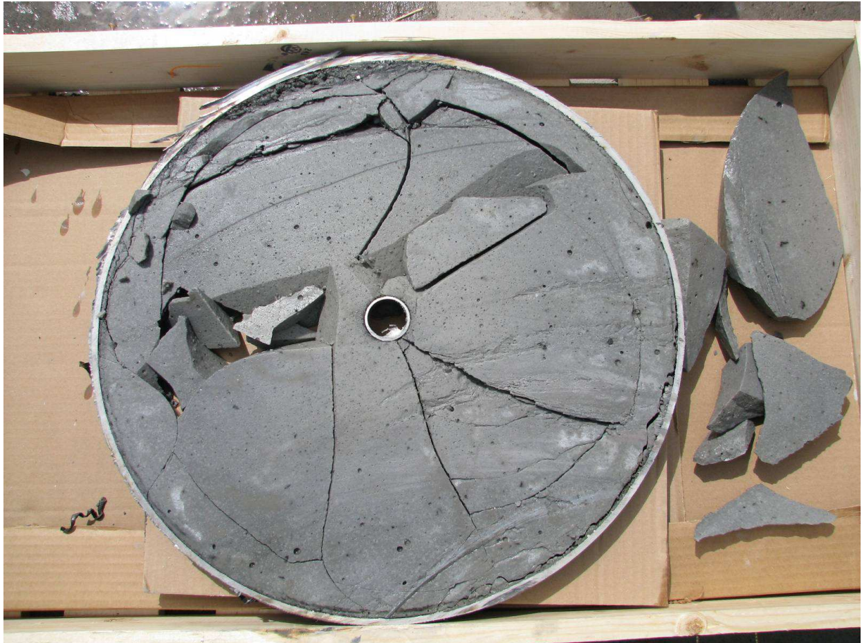
Fig.12. Cracking in the mid-plane in CWF1
