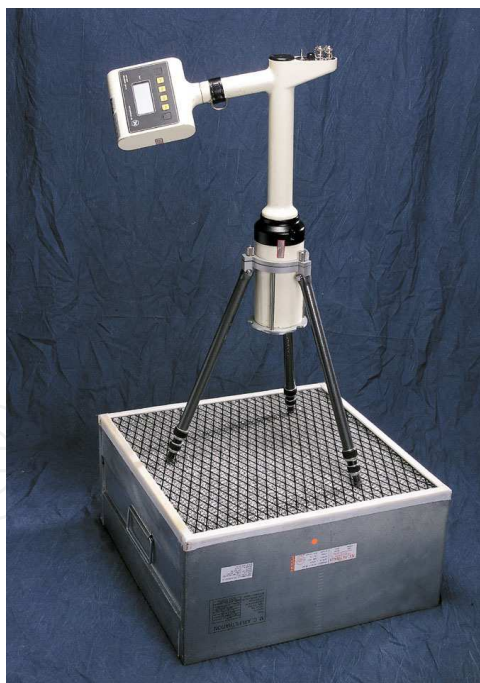
Fig. 2. LRGS positioned for HEPA filter monitoring
