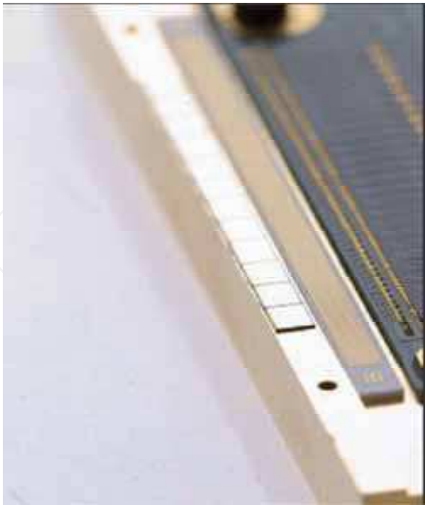
Fig. 17. Photograph of a DLAM ‘super-array’ comprising a number of monolithic array chips bonded on a common carrier, with the pitch between arrays maintained across the entire print head.
