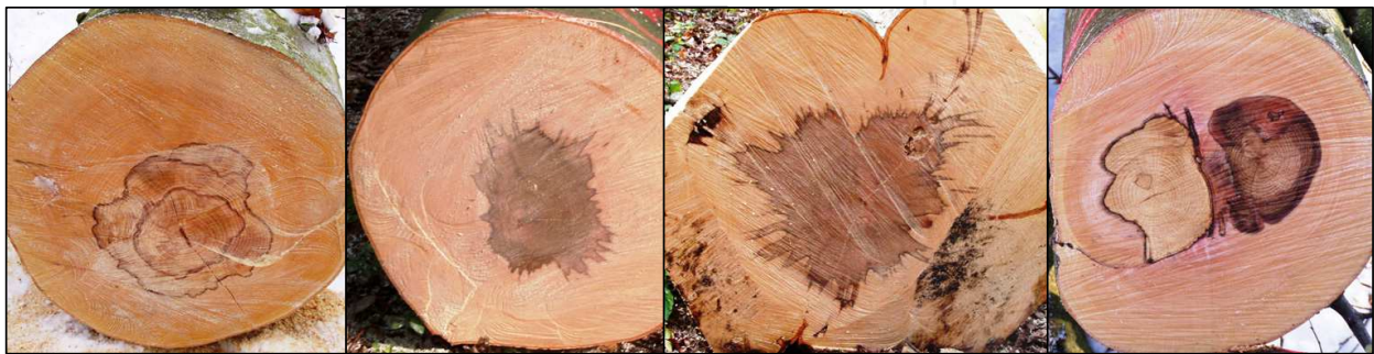
Fig. 2. Different shape of beech false heartwood
