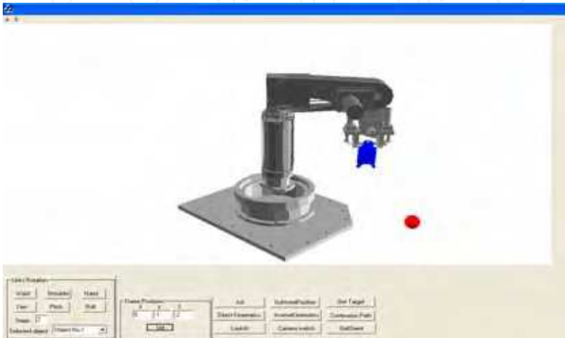
Figure 2. Schematic view of simulator software designed for 6R robot
