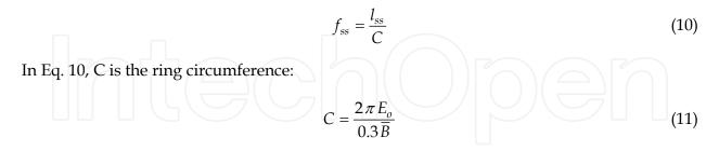
In Eqs. 9 – 11, v is the muon velocity,  $l_{ss}$  is the straight section length,  $E_o$  is the muon energy,  $\overline{B}$  is the ring's average magnetic induction, and N is the number of muon decays in a year.
