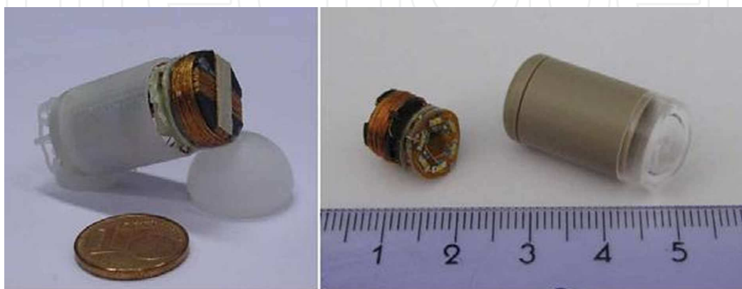
Fig. 3. 3D coil inside capsule endoscope for wireless power transmission (Carta et al. , 2010).
