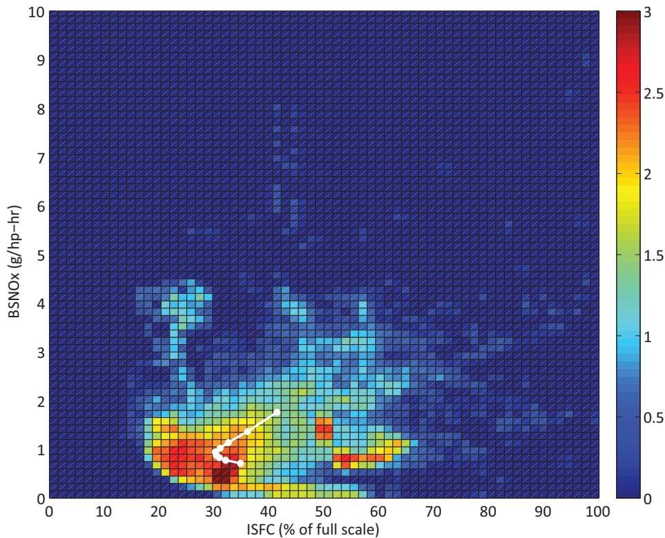
Fig. 14. Distribution of (ISFC, BSNO<sub>x</sub>) pairs for the oxygen concentration based fueling controller
