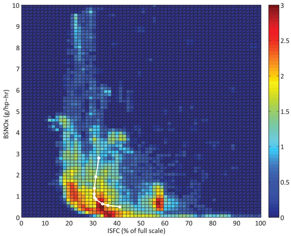
Fig. 15. Distribution of (ISFC, BSNO<sub>x</sub>) pairs for the conventional fueling controller
