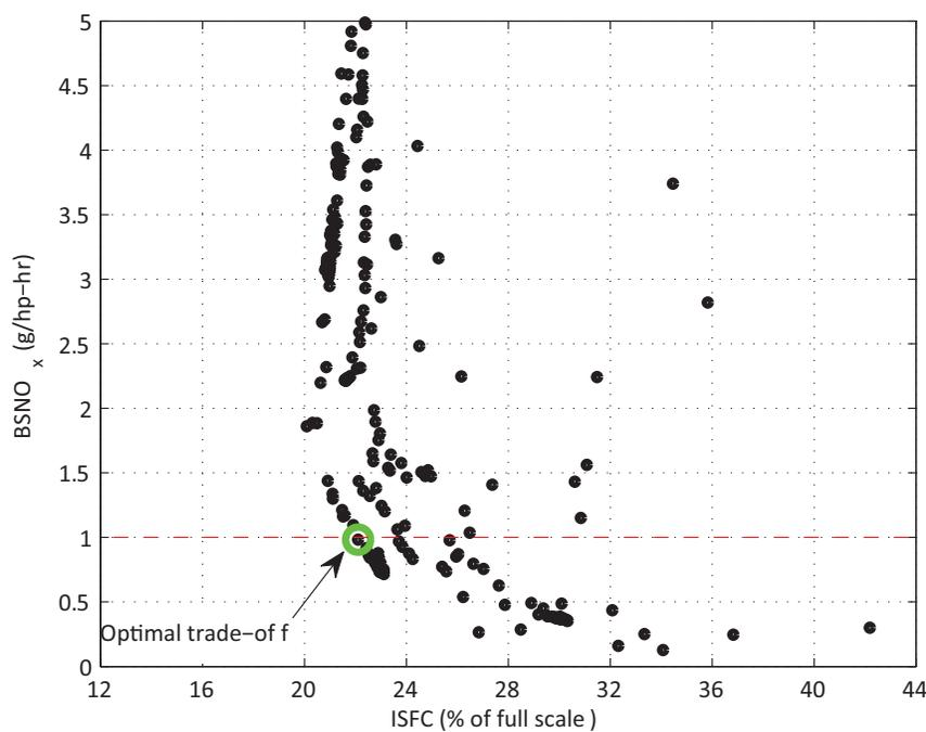
Fig. 5. Fueling parameter calibration example (1000 RPM, 65 mg fuel)
