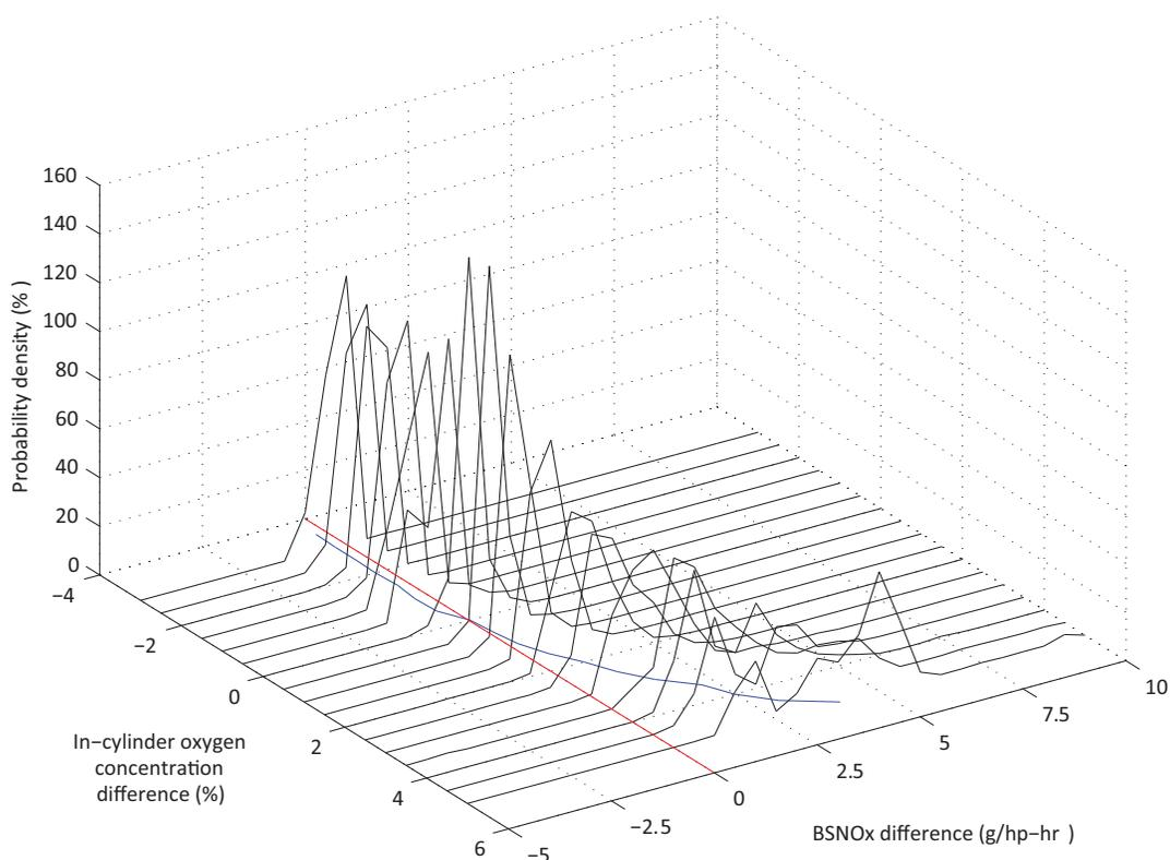
Fig. 13. Instantaneous BSNO<sub>x</sub> difference (Conventional - [O<sub>2</sub>]<sub>cyl</sub> based) probability density functions
