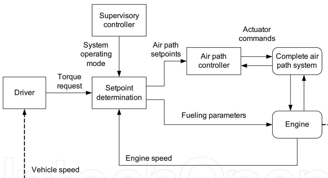
Fig. 1. Current approach to diesel engine control
