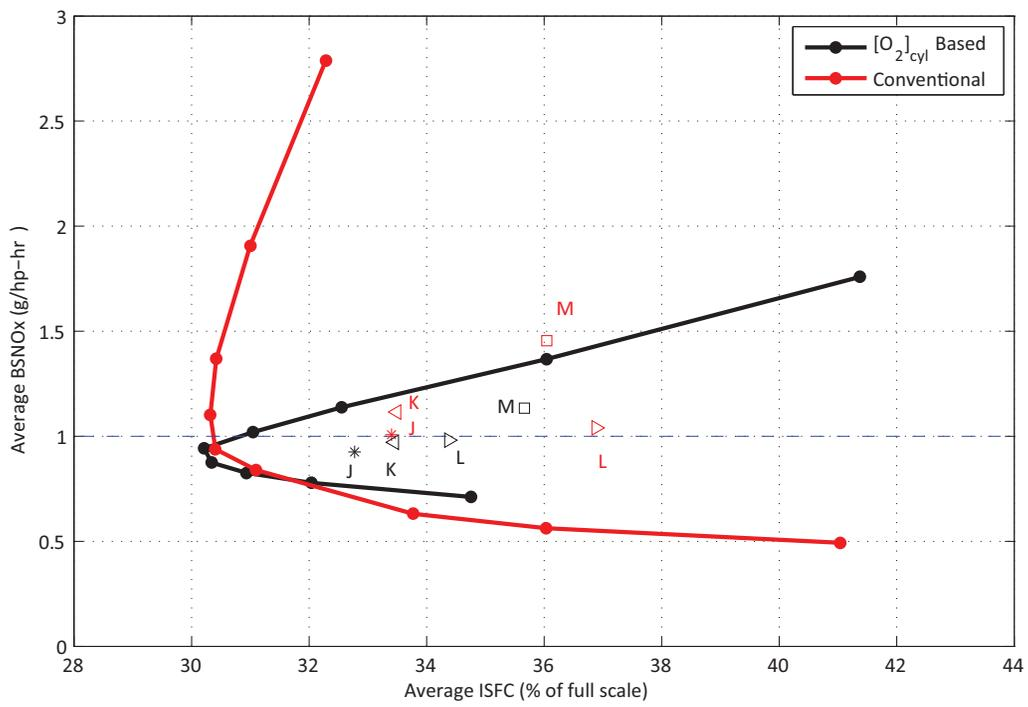
Fig. 16. Trade-off between cycle averaged BSNO<sub>x</sub> and cycle averaged ISFC: Dynamic air path errors
