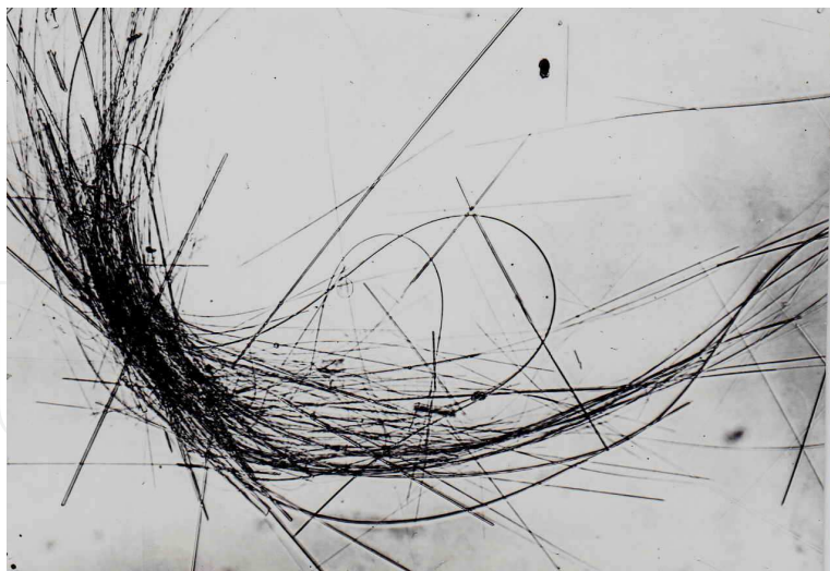
Fig. 10. Micrograph of synthetic fibrous fluorosilicates (x 110).
