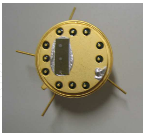
Fig. 8. Photograph of three hydrogen sensors bonded on a header.
