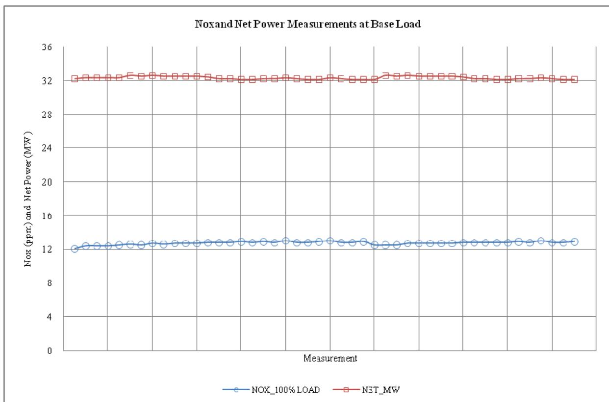
Fig. 7. NO<sub>x</sub> measurements (ppm) and Net Power (MW) recorded during test at 100% load.
