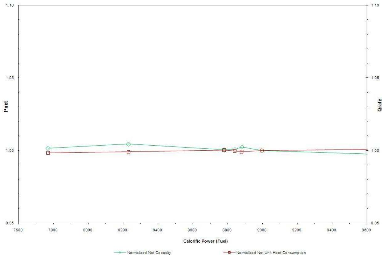
Fig. 6. Correction curve by calorific value of fuel.
