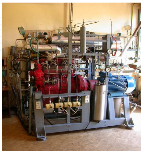
Fig. 8. Д-245 diesel-based synthesis gas generator.
