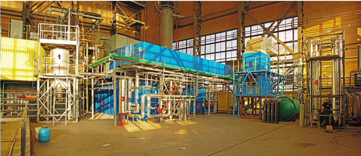
1 - The synthesis gas generator by partial gas oxidation with syngas cooler, 2 - gas turbine, 3- soot filter, 4 - water heating boiler, 5 - water cooling tower, 6 - block of methanol synthesis.
