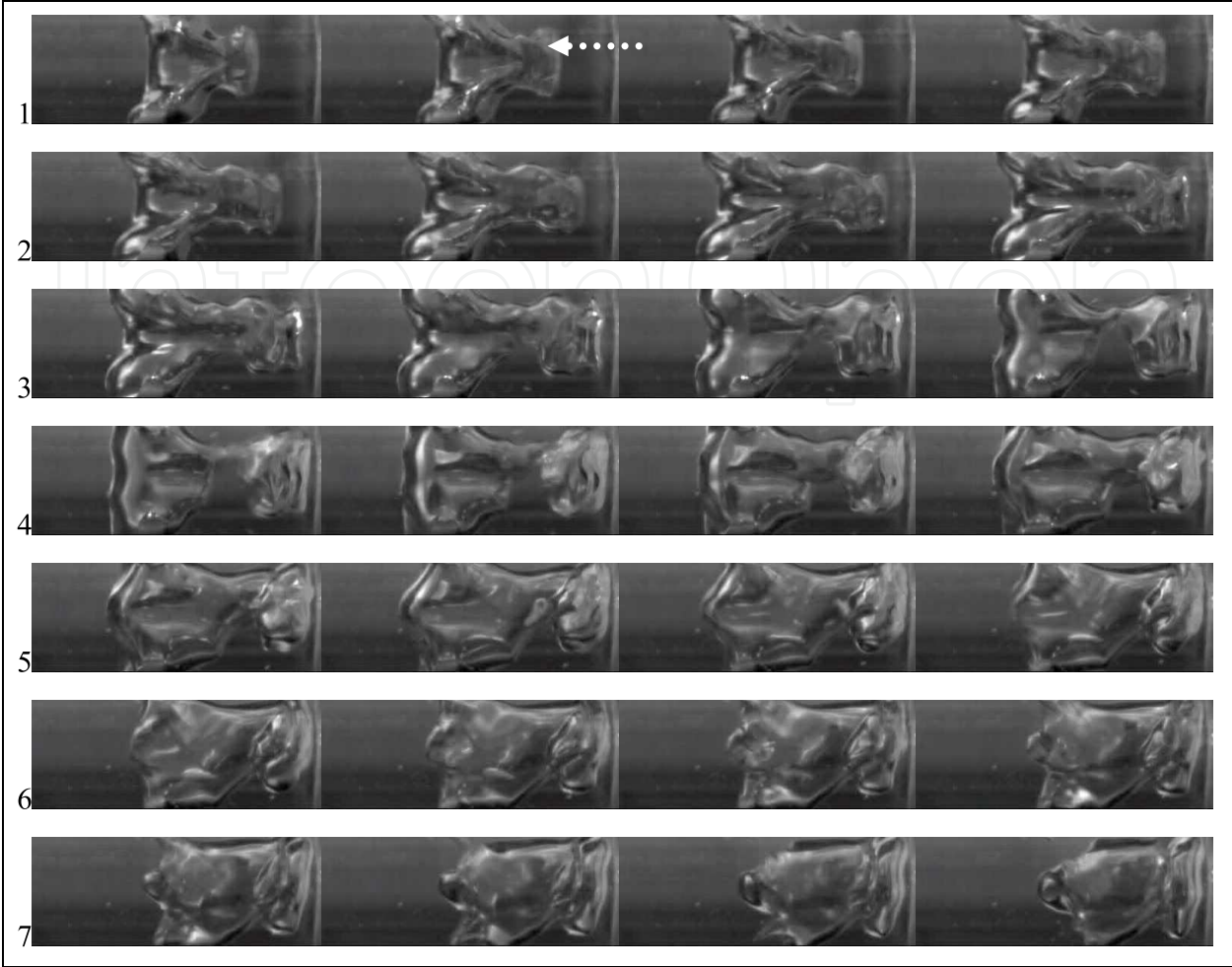
Fig. 10. Images of the process of bubble collapse at \gamma \approx 3 . The peak strength of the pressure wave is 300kPa. The size of each individual frame is 9.6 mm \times 3.1 mm. R_{\max} : 2.35 mm. The image time interval is 1/4000 second. (The Kelvin -Helmholtz vortex is indicated by a dotted line with an arrow).
