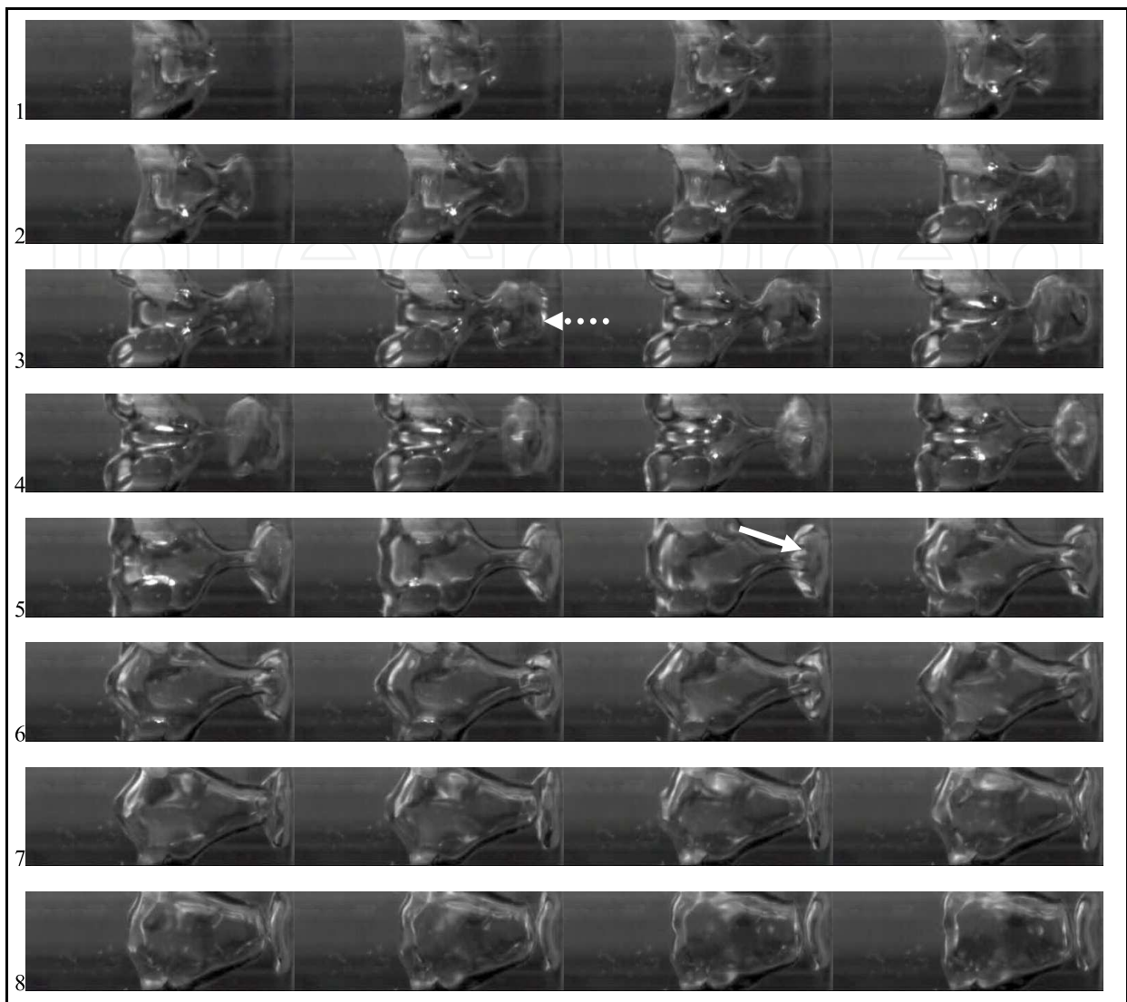
Fig. 11. Images of the process of bubble collapse at \gamma \approx 3 . The peak strength of the pressure wave is 365 kPa. The size of each individual frame is 2.25 mm. The image time interval is 1/4000 second. (The Kelvin-Helmholtz vortex is indicated by a dotted line with an arrow; the counter jet is indicated by a solid line with an arrow).
