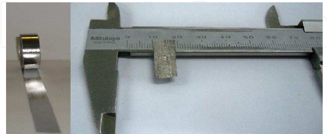
Fig. 13. \text{Fe}_{78}\text{Si}_{13}\text{B}_9 amorphous strips used in magnetic cores, and industrial magnetic package.
