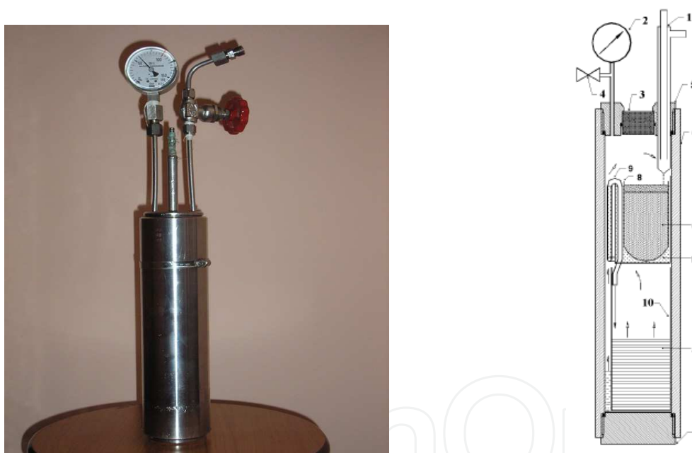
1) Cooling finger; 2) Pressure gauge; 3) Sapphire Window; 4) Valve; 5) Upper cover; 6) Steel Cylinder; 7) Bottom cover; 8) Extracting thimble; 9) Siphon; 10) Product dropping glass; A) Product; B) Extract solution; C) Plant material
