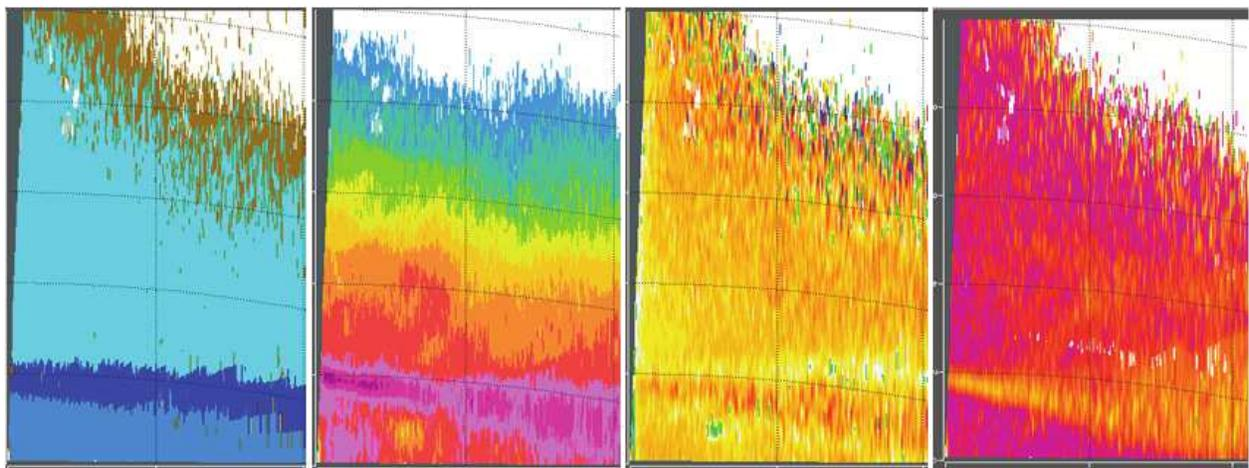
Fig. 5. RHI scans north of Vantaa radar 30 August 2009 00:45 UTC. . Range 100 km, height 10 km, parameters from left to right: Hydrometeor classification, reflectivity  $Z$ , differential reflectivity  $ZDR$  and copolar correlation factor  $Rho_{HV}$ .
