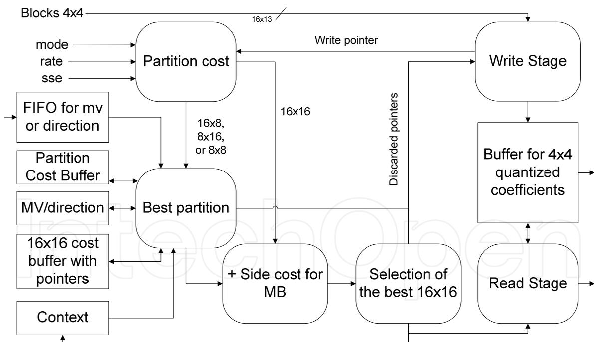
Fig. 13. Block diagram of the mode selection module
