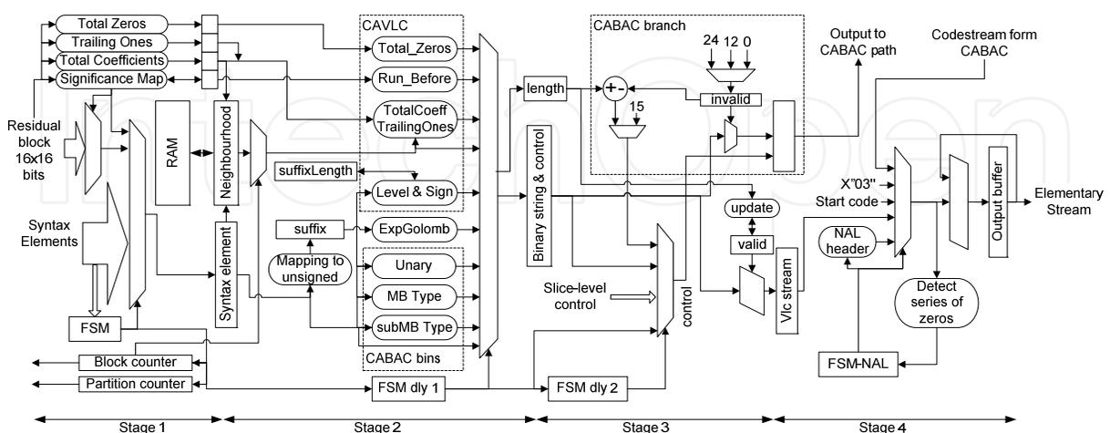
Fig. 14. Block diagram of the double-mode binarization unit
