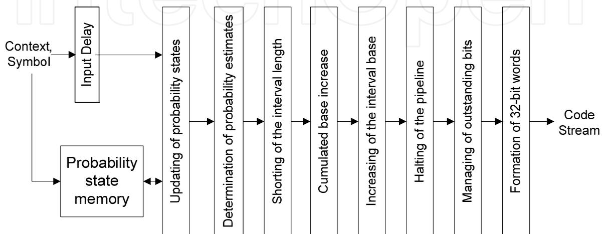
Fig. 16. Arithmetic Coding Pipeline
