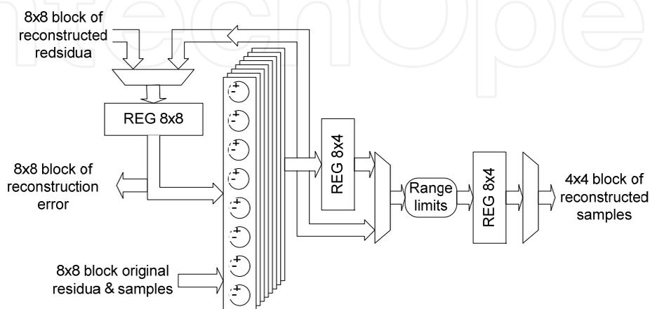
Fig. 12. Block diagram of the reconstruction unit
