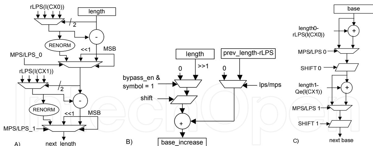
Fig. 17. Arithmetic Coding Stages 4th-6th
