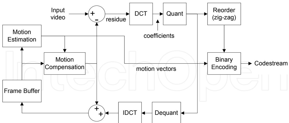
Fig. 1 Block diagram of the video encoder
