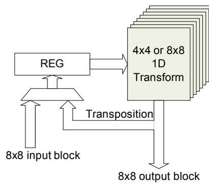
Fig. 10. Block diagram of the transform module
