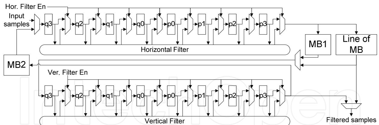
Fig. 18. Dataflow in the deblocking filter
