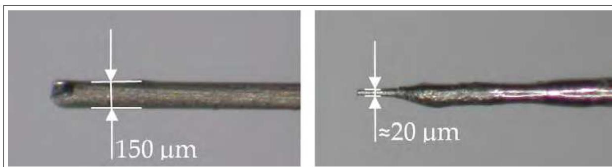
Fig. 30. Tool before (diameter 150  $\mu$ m - left) and after the tooling process (diameter  $\approx$ 20  $\mu$ m - right)
