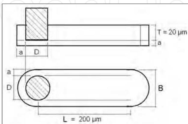
Fig. 12. Sketch of the produced groove
