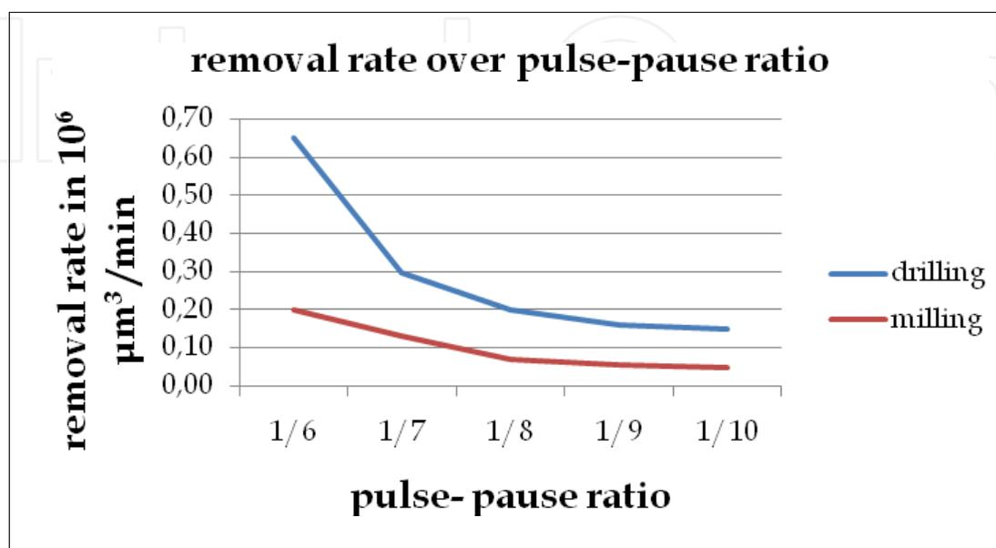
Fig. 27. Removal rate over pulse-pause ratio
