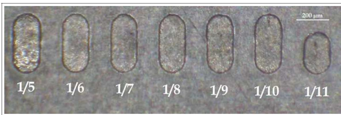
Fig. 26. Grooves produced for the pulse-pause ratio experiment
