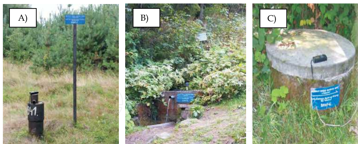
Fig. 2. Types of monitoring points: A) Piezometer, B) Spring, C) Well. (Sources of photos: Glubiak-Witwicka et al., 2003)
