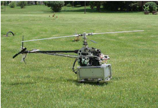
Fig. 2. Implemented ServoHeli-20 RUAV
