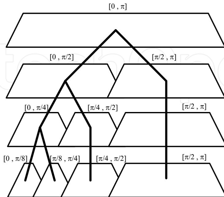
Fig. 8. Frequency Spectrum of a three-stage Subband Structure
