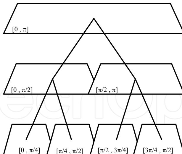
Fig. 13. Frequency Bands of Mallat's 2-D Analysis Algorithm
