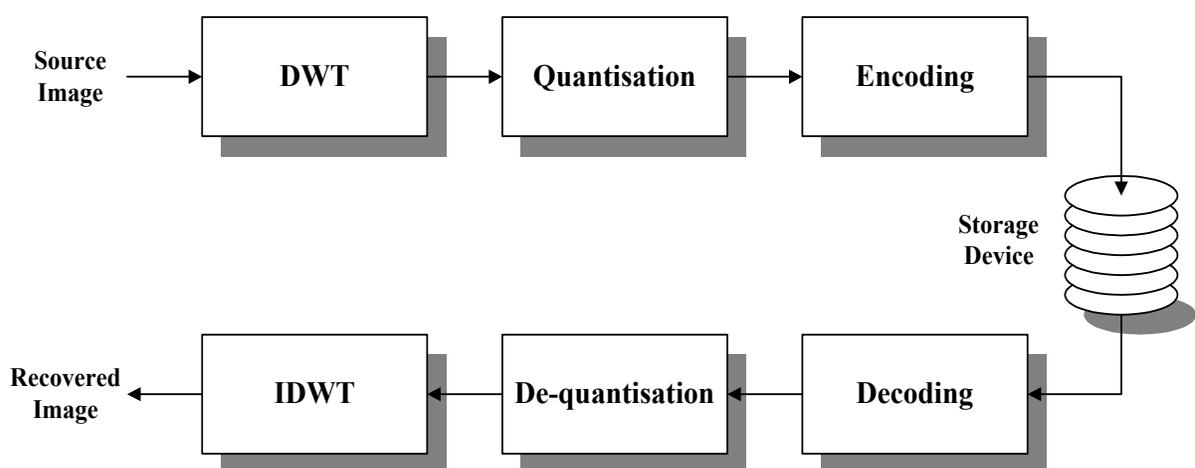
Fig. 21. Wavelet-based encoding scheme
