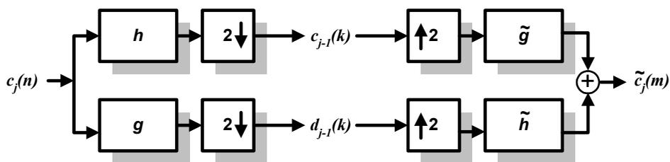
Fig. 18. Two-band analysis and synthesis filter bank
