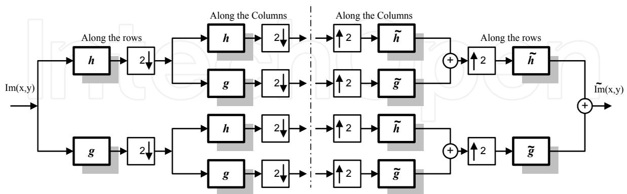
Fig. 12. Two-dimensional Mallat's analysis and synthesis tree
