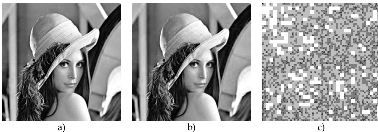
Fig. 2. An example of image denoising using a bandelet transforms. a) Original image, b) Denoised image using a bandelet transforms, and c) Dyadic squares tree
