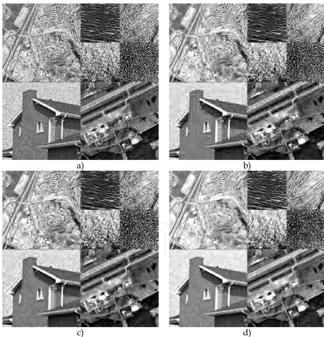
Fig. 11. a) Original speckled image, b) Despeckled image obtained with the original bandelet denoising scheme, c) Despeckled image obtained with the original contourlet denoising scheme, and d) Despeckled image obtained with the MBD denoising technique
