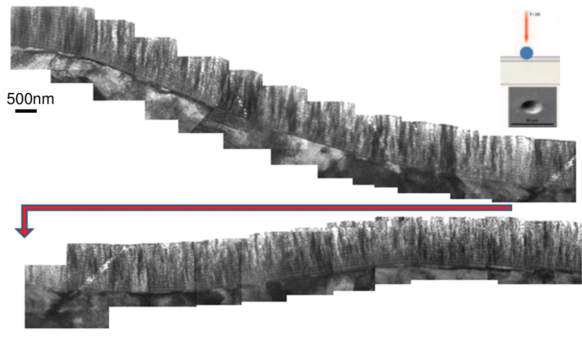
Fig. 12. Microstructure analysis of multilayered Ti/TiN coatings after static mechanical test done on a cross- section by TEM technique.
