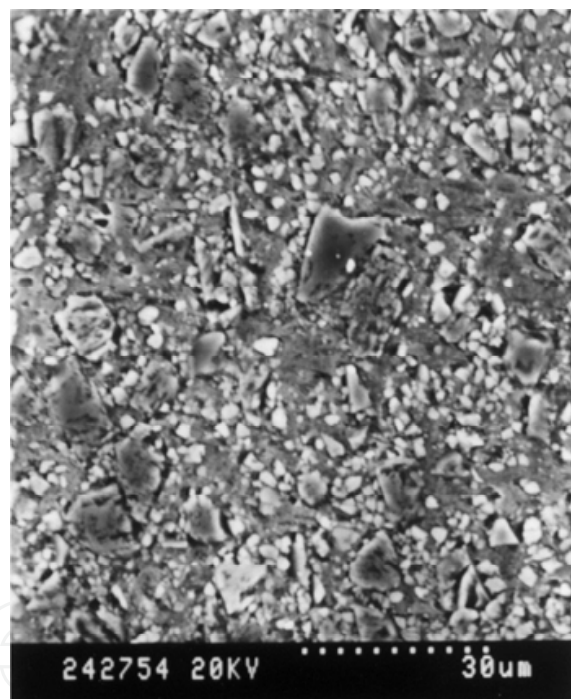
Fig. 1. Microstructure of aluminum matrix composite \text{SiC}_p/\text{A356}
