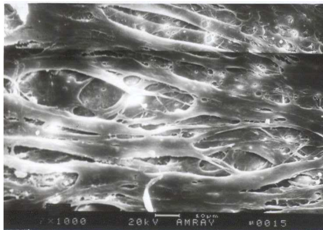
Fig. 3. The compound of osteoblast cells and the material (scanning electron microscope, 1000×)
