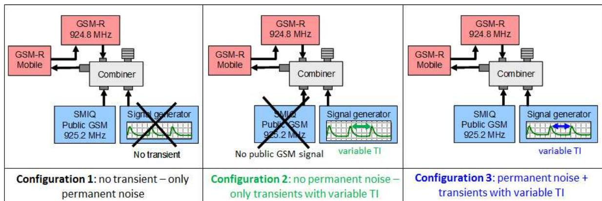
Fig. 10. The different configurations used for immunity testing
