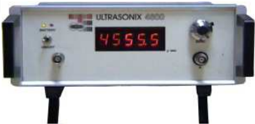
Fig. 6. Compressional wave velocity (P-wave) measuring device 'Ultrasonix 4600'
