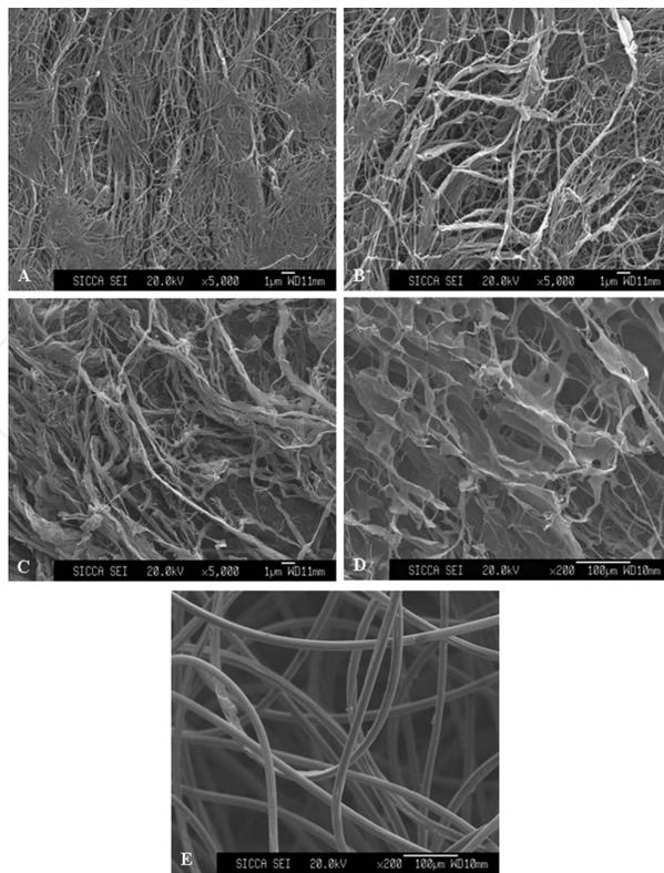
Fig. 5. EMS examination of different materials' surface. (A) urethral surface of ACSM, EMS $\times$ 5,000, (B) cavernosal surface of ACSM, EMS $\times$ 5,000 (C) surface of BAMG, EMS $\times$ 5,000. (D) surface of SIS, EMS<sub>200</sub>. (E) surface of PGA, EMS $\times$ 200.
