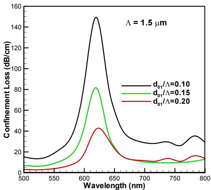
Fig. 6. Loss spectra of proposed PCF SPR biosensor in the vicinity of the first plasmonic peak for variation in  $d_{01}$ . Analyte refractive index ( $n_a=1.33$ ),  $t_{Au} = 40$  nm,  $d_1/\Lambda = 0.20$ ,  $d_2/\Lambda = 0.35$ .
