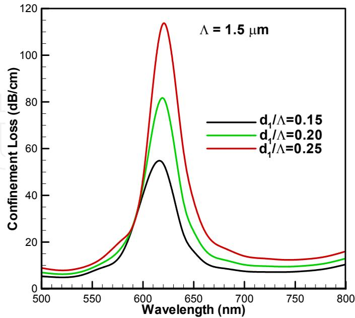
Fig. 4. Loss spectra of proposed PCF SPR biosensor in the vicinity of the first plasmonic peak for variation in  $d_1$ . Analyte refractive index ( $n_a=1.33$ ),  $d_{01}/\Lambda = 0.15$ ,  $t_{\text{Au}} = 40 \text{ nm}$ ,  $d_2/\Lambda = 0.35$ .
