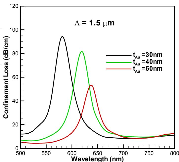
Fig. 3. Loss spectra of proposed PCF SPR biosensor in the vicinity of the first plasmonic peak for variation in gold layer thickness ( $t_{Au}$ ). Analyte refractive index ( $n_a=1.33$ ),  $d_{01}/\Lambda = 0.15$ ,  $d_1/\Lambda = 0.2$ ,  $d_2/\Lambda = 0.35$ .
