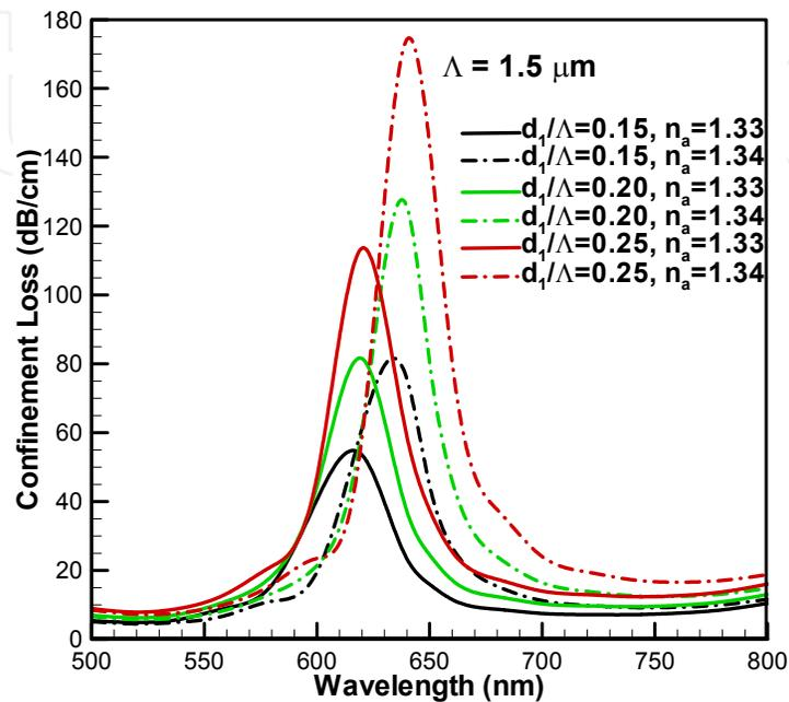
Fig. 9. Shift in resonant wavelength of the loss spectrum for a variation in  $d_1$  of the proposed SPR sensor. Analyte refractive index ( $n_a=1.33$ ),  $d_{01}/\Lambda = 0.15$ ,  $t_{\text{Au}} = 40 \text{ nm}$ ,  $d_2/\Lambda = 0.35$ .
