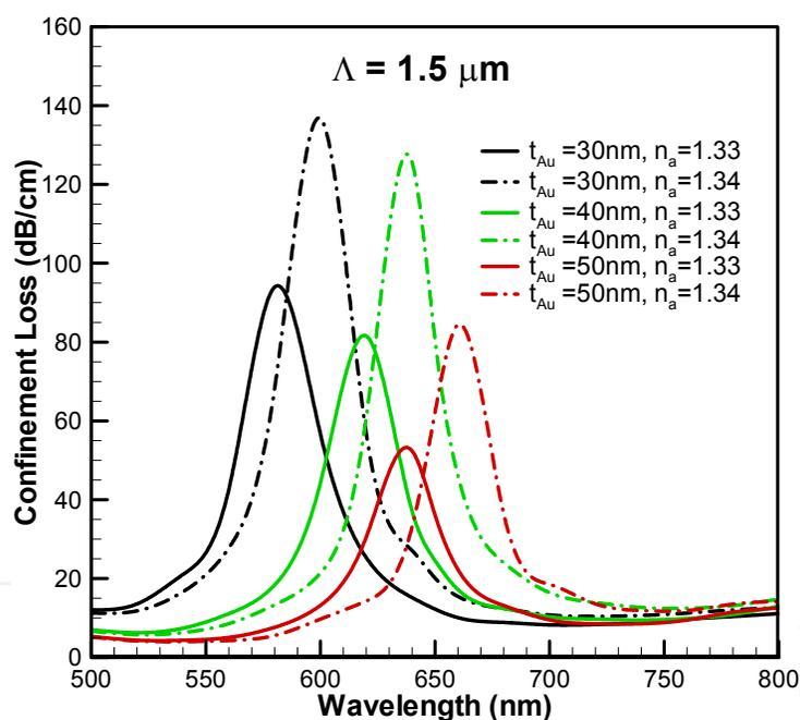
Fig. 8. Shift in resonant wavelength of the loss spectrum for a variation in  $t_{Au}$  of the proposed SPR sensor. Analyte refractive index ( $n_a = 1.33$ ),  $d_{01}/\Lambda = 0.15$ ,  $d_1/\Lambda = 0.2$ ,  $d_2/\Lambda = 0.35$ .
