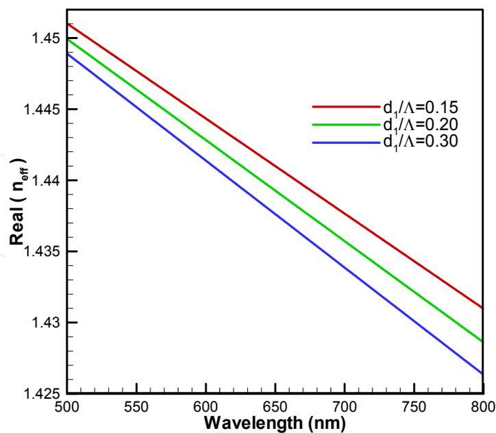
Fig. 5. Dispersion relation of the fundamental mode for variation in  $d_1$ . Analyte refractive index ( $n_a=1.33$ ),  $d_{01}/\Lambda = 0.15$ ,  $t_{\text{Au}} = 40 \text{ nm}$ ,  $d_2/\Lambda = 0.35$ .
