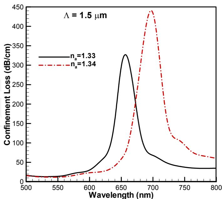
Fig. 10. Shift in resonant wavelength of the optimised PCF SPR biosensor. Structural parameters;  $\Lambda = 1.5 \mu\text{m}$ ,  $d_1/\Lambda = 0.50$ ,  $d_{01}/\Lambda = 0.20$ ,  $t_{\text{Au}} = 40 \text{ nm}$ .
