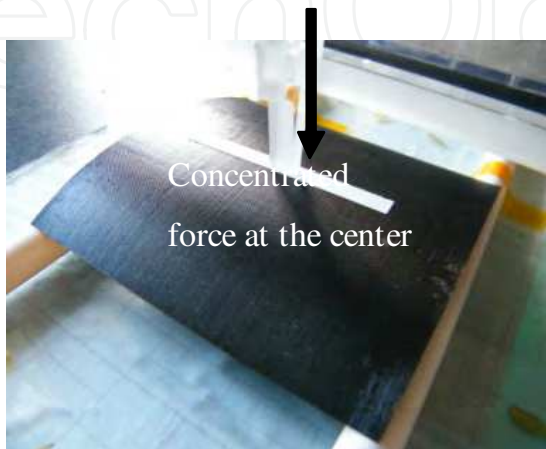
Fig. 3. Schematics of concentrated force load experiments
