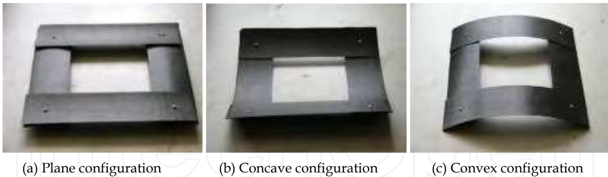
Fig. 10. Three stable configurations of lattice structures
